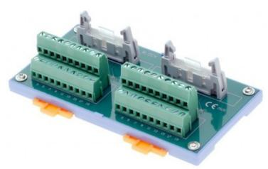
Double terminal board with 2 x 20 screw terminals 2 x 20 pole IDC male connector For DIN rail mounting Incl. x 1m flat cable IDC20 female to IDC20 female 148 x 70 mm (W x L)
